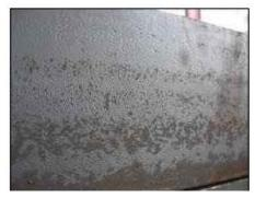
IMPORTANT: It is imperative that all mill scale, raised and loose flaking rust is sanded off so that it is very smooth to prevent moisture ingress and/or rusting under the coating. Mill scale, further rusting and moisture ingress will cause the coating to lose adherence causing discolouration and lifting.
